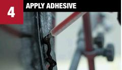
Apply 3/8" - 1/2" bead of **Dual-Mix™ Multi-Purpose Panel Adhesive or Dual-Mix Weld-Bond Adhesive** to both surfaces. Use enough material to completely fill the joint when parts are clamped. Tool with a spreader or acid brush. Cover all exposed bare metal.
