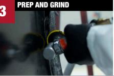
Clean with SEM Solve or XXX Universal Surface Cleaner. Grind mating flanges with a 36 grit grinding disc at low speed for aggressive grind mark. Remove any adhesive or protective coatings.
