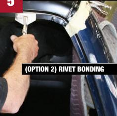
Clamp panel into place. Do not over clamp. Wipe away excess material.
